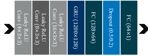
Fig. 10. Flow rate estimator architecture.
